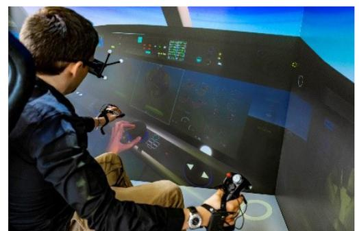
Collaboration between reviewers is enhanced using side display platforms. This specific platform displays the point of view of the immersed user, or another point of view on the scene being experienced. The immersed user is provided with a user-friendly immersive menu and has access to VR-review dedicated tools (navigation, configuration control, cut plane, etc.)
